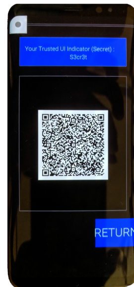
Figure 5: Registering with the bank by showing the QR code of public key on the trusted screen
