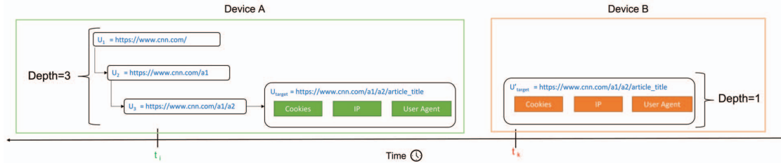
Figure 4: Session reconstruction. The timeline of events represents the intuition of our approach. First, a device (A) is visiting a web site at time t_i and is generating a series of actions in order to access U_{target} through a URL path that connects U_1 to U_3 . At a later time, t_k , a different device (B) is accessing U'_{target} , but without issuing HTTP requests for any of the intermediate steps of the path U_1 to U_3 . This action, thus, is signaling an event that the second session, initiated at t_k , is a synced session.
