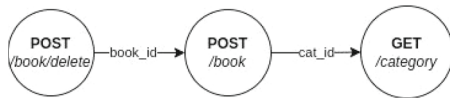
Fig. 5 An example of the dependency graph model. The get category API will produce a cat ID that will be needed for calling the post book API. The latter will generate a book ID used by the delete book API
