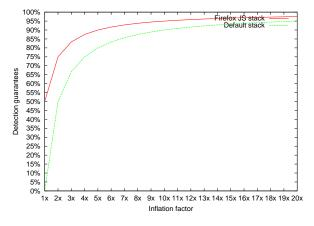
Figure 2: Effect of stack spraying (JS-visible or default stack) on our detection guarantees (DGs) across different inflation factors.
